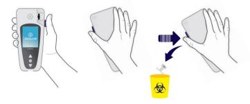
To minimize the risk of contamination, this unique ejection system was designed such as user never gets in contact with a used SmartChip.
