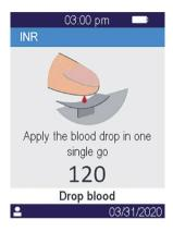
Prick the side of a fingertip of the patient. A minimum volume of  $3\mu$ L of blood is required to fill the central micro channel. Do not squeeze the finger, as this may lead to incorrect results.
