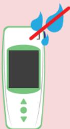
Make sure not to drop any liquid in the Tsmart® insertion area; if this occurs, do not use the device and immediately contact your reseller.
