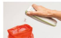
1 Insert the Tsmart® INR microcuvette into the LabPad® INR: the device switches on automatically.
