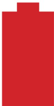
When a red battery is displayed full-screen, it means the battery charge is critical and the device will automatically switch off.
