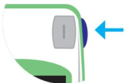
The side blue button releases the Tsmart<sup>®</sup> INR for discarding after use (see [section 5.5 Discarding the microcuvette](#)).
