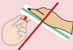
Do not try to pull the Tsmart<sup>®</sup> INR, as you may damage the microcuvette and leave part of it inside the device.
