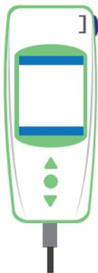
The LabPad® INR can be operated on battery or from an electrical power supply. For the latter, connect the provided cable to the micro USB port located on the lower part of the device and the battery charger (power adapter) to a power supply. The provided cable complies with CEI 61010 standard.
